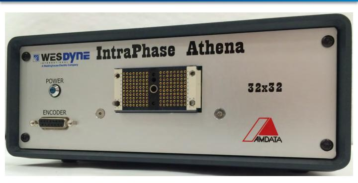
The Athena 32/32 Phased Array system, manufactured by WesDyne NDE Products & Technology, consists of a phased array acquisition system and personal computer running standard IntraSpect software. The PC is a full featured computer that performs the acquisition, analysis and storage of the data. The system hardware is capable of operating up to four data sets with any combination of phased array or conventional UT probes.
