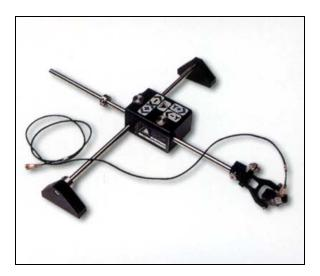
A Model 4020 scanner shown above with an angle beam transducer and UT cable (scanner encoder cable not shown). Encoders are contained within the black box shown in center of photo. Rods slide through the box in both X and Y directions as an operator manually moves the transducer over an inspection surface, providing encoded positional feedback with the UT signal for pulse-on-position style ultrasonic imaging.
