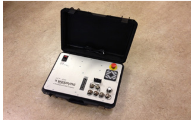
Example of an MCP design: type and layout depend on connector interface needs and system capabilities (number of axes, manipulator-specific design, etc.).
