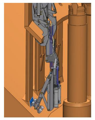
Configuration for sizing of defect using time-offlight diffraction (TOFD)
