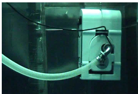
U-DEC system cleaning cavity walls
