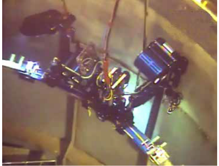
DUIT in mockup reactor performing inspections
