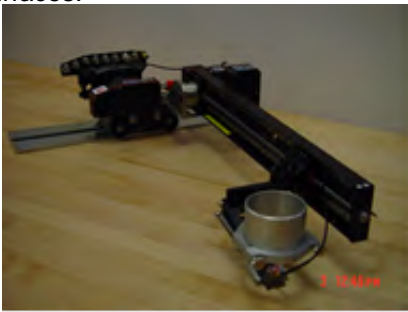
5085 scanner in a standard configuration, shown without cabling attached. Shown with manual skewing collar and spring loaded gimbaling.
