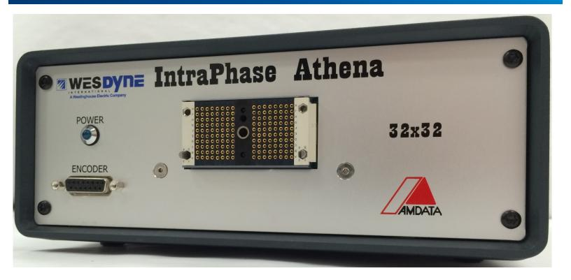
The Athena 32/32 Phased Array system, manufactured by WesDyne NDE Products & Technology, consists of a phased array acquisition system and personal computer running standard IntraSpect software. The PC is a full featured computer that performs the acquisition, analysis and storage of the data. The system hardware is capable of operating up to four data sets with any combination of phased array or conventional UT probes.
