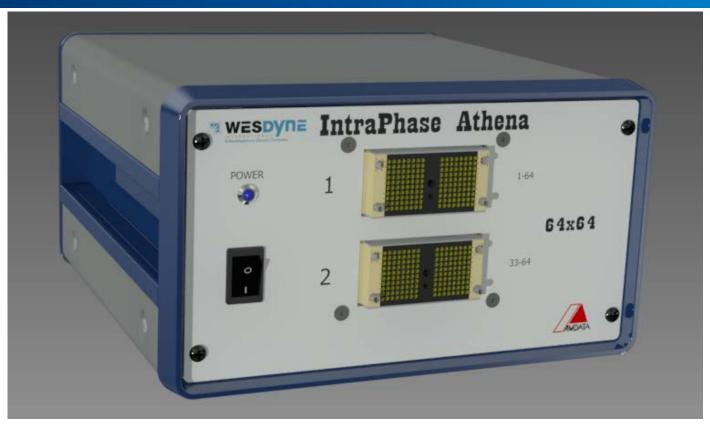
The Athena 64/64 Phased Array system, manufactured by WesDyne NDE Products & Technology, consists of a phased array acquisition system and personal computer running standard IntraSpect software. The PC is a full featured computer that performs the acquisition, analysis and storage of the data. The system hardware is capable of operating up to four data sets with any combination of phased array or conventional UT probes.
