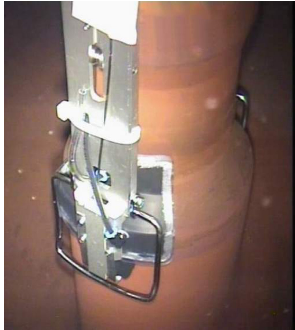
MouldMan tooling applied on emergency nozzle during A-VT inspection for defect height sizing.
